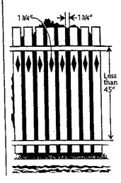
If the distance between the tops of the horizontal members is more than 45 inches, the horizontal members can be on the side of the fence facing away from the pool. The spacing between vertical members should not exceed 4 inches. This size is based on the head breadth and chest depth of a young child and is intended to prevent a child from passing through an opening. Again, if there are any decorative cutouts in the fence, the space within the cutouts should not exceed 1-3/4 inches.
