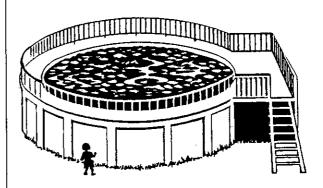
Aboveground pools should have barriers. The pool structure itself serves as a barrier or a barrier is mounted on top of the pool structure.
