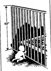
Guidelines recommend eliminating handholds and footholds and minimizing the size of openings in a barrier's construction. For a Solid Barrier: No indentations or protrusions should be present, other than normal construction tolerances and masonry joints.
