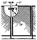
Also, the gate and barrier should have no opening greater than 1/2 inch within 18 inches of the latch release mechanism. This prevents a young child from reaching through the gate and releasing the latch.
