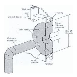
Listed solid fuel pre-fabricated metal chimneys can also be used to pass through a combustible wall when installed according to manufacturers' recommendations.
