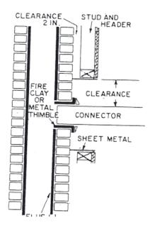
Try to avoid passing a connector pipe through an interior wall. If this must be done, use a ventilating thimble (See Figure 4). The thimble diameter must be at least 12 inches larger than that of the stovepipe, thus giving at least 6 inches of metal-lined, ventilated clearance. It you do not use a thimble, the clearance must be three times the pipe diameter. A 6 inch pipe would need a 42 inch diameter hole cut through a combustible wall.
