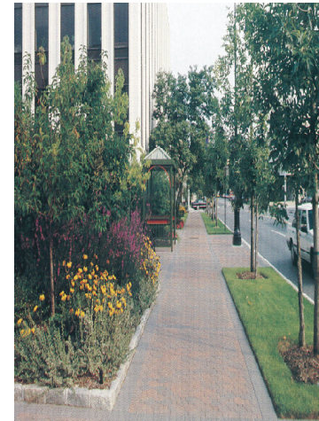
fig 5-1: Sidewalk Buffer for Vehicle Overhang
