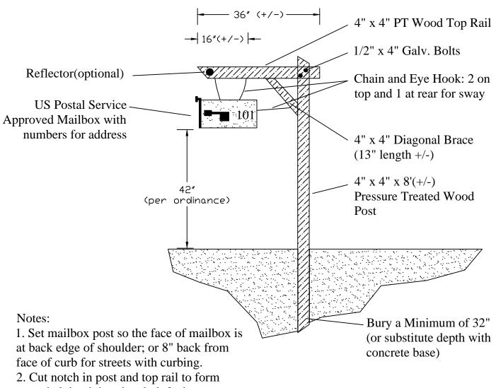
2. Cut notch in post and top rail to form cross-halving joint, then bolt 2 pieces together.
