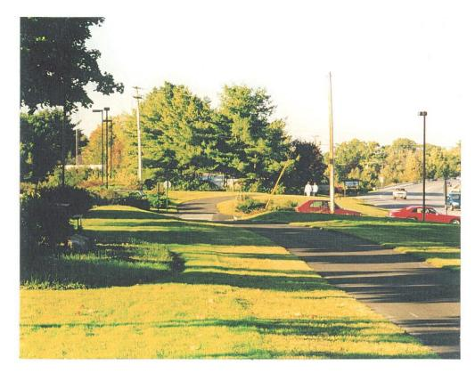
Bituminous concrete pathways should be carefully designed and detailed. Note signage used at crosswalks. Driveway grade was adjusted to meet ADA requirements for crosspitch on crosswalks.
