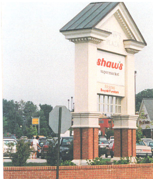
An appropriate project identification sign, scaled to the space and building that it advertises. The details, lettering styles, and colors are all derived from the architecture.
