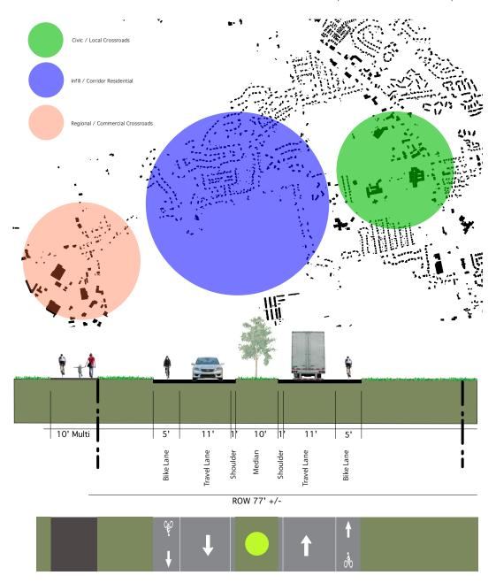
The Town of Scarborough retained the team of Woodard & Curran and MRLD to develop a Complete / Green Street preliminary design for a three-mile stretch of Gorham Road. The design builds off previous studies such as the Transportation Master Plan and the Comprehensive Plan, but fine tunes site specification recommendations for streetscape, mobility, access management, Complete Streets, and green infrastructure – including a new state of the art Nonesuch River stream crossing.
