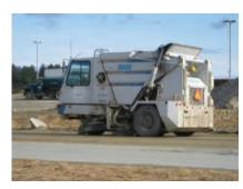
**Sweep and Vacuum** paved road surface when dry. Sweep from the center line to the edge of the travel way. Do not sweep into a waterbody or wetland. The public roadway may also require sweeping.
