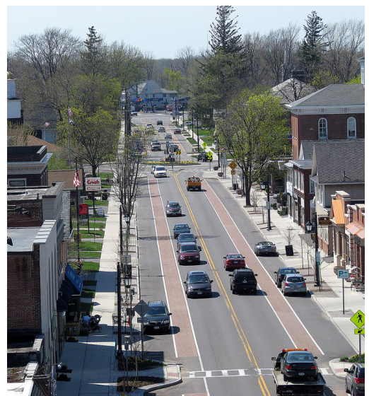
This main street from Hamburg, NY is built for all users, from pedestrians, to cyclists, to motorists looking for on-street parking to access shops and restaurants along the roadway. (Photo credit: Flickr, Complete Streets Coalition)
