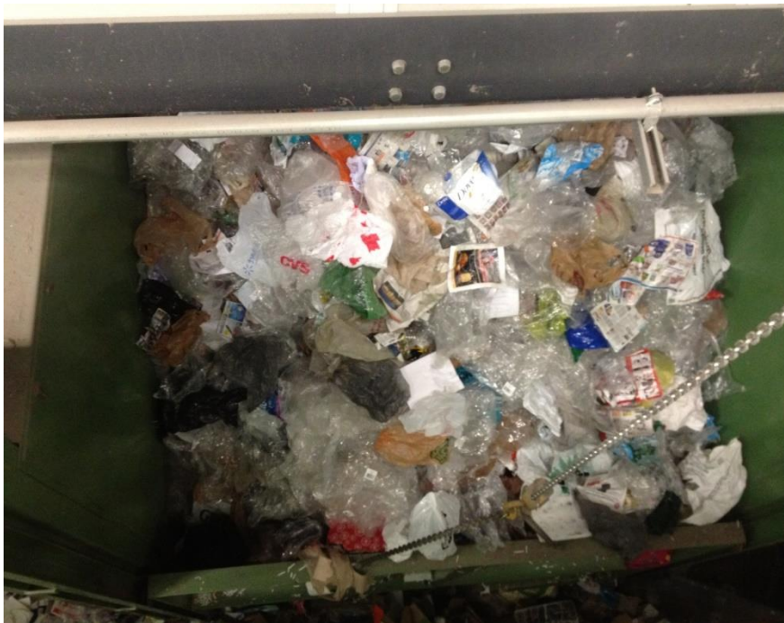
“And the last photo is of the composition of our bypass bay. The bay is where we put all the trash that comes in with the recycling. Typically our bypass rate is running somewhere between 6% and 8%. The majority of that as you can see, is plastic film.” Leo Maheu—ecomaine
