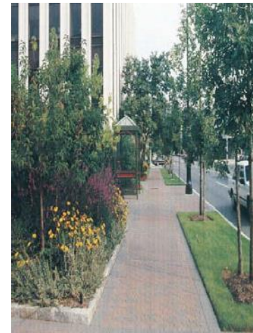
fig 5.1: Sidewalk Buffer for Vehicle Overhang
