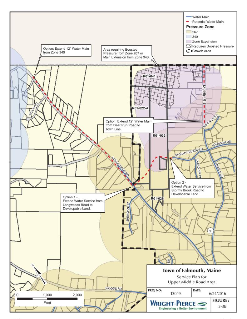
A more detailed study is needed to develop a service plan for this area if this option is desired. The PWDs policy towards installation of booster pumping stations is discussed later in the report. This approach will be less costly then extending a new water main from Zone 340. The estimated cost for a booster pumping station is approximately \$500,000 for a buried capsule style station
